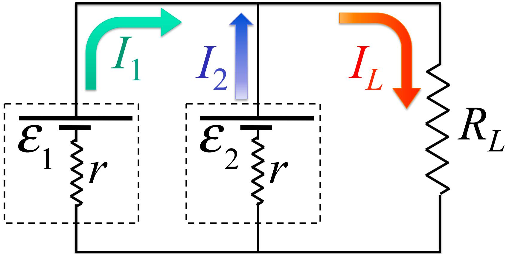
$$I_L = \frac{\mathcal{E}_1 + \mathcal{E}_2}{2R_L + r}, \text{ if } \mathcal{E}_1 = \mathcal{E}_2 = \mathcal{E}, \text{ then } I_L = \frac{2\mathcal{E}}{2R_L + r} = \frac{\mathcal{E}}{R_L + r/2}$$
